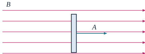
(a) B is along the normal, so the flux is a maximum, BA
